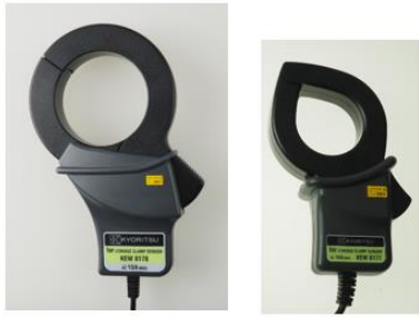
Automatic identification of the current sensors
