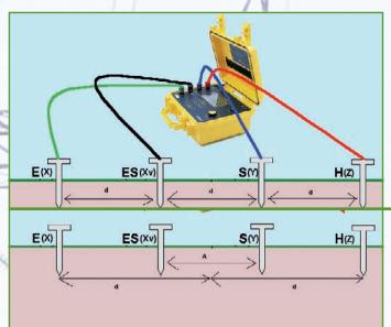
**Wenner method:** the distances between the 4 rods are identical:  $d \rho W = 2.\pi.d.R_{SSE}$
